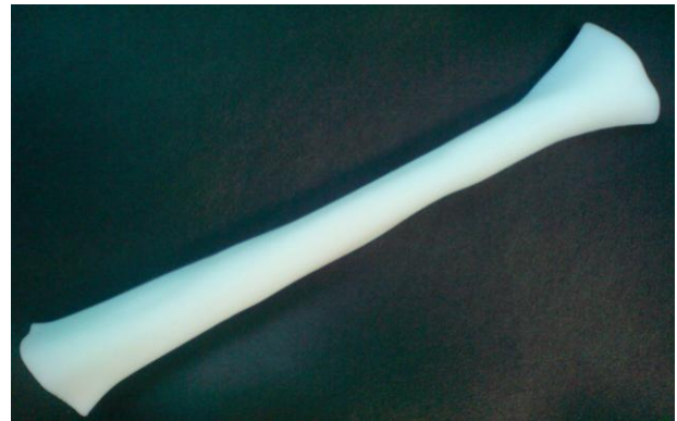
Fig .5.2.3 RPT Model of Humerus Bone Using ABS material
